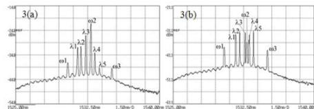
Fig. 1. EDFRL generated spectrum which produced multi wavelength through the experimental setup with PCF ZDW at (a) 1550 nm and (b) 1040 nm
