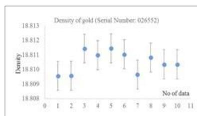
Figure 4 : Measurement results of gold density using hydrostatic weighing method
